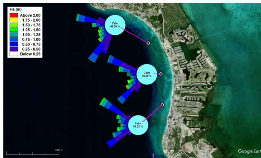
**Figure 8-4 Simulated wave roses along the 5m depth contour, period : (2010-2022).**
