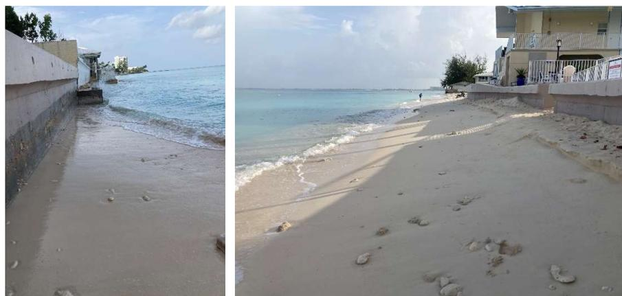
**Figure 1-2 Severe beach erosion at Cayman reef resort, 2023. On the right photo the location of the water line during a recent high-water event can be noticed.**
